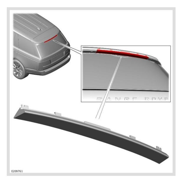
The High Mounted Stop Lamp (HMSL) is located above the rear window. The lamp comprises a plastic housing with a red coloured lens. The lamp is illuminated by Light Emitting Diodes (LED).
