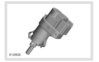
The stop lamp switch is a two pole switch mounted in the brake pedal bracket and operated by the brake pedal. The output connections of the two poles are hardwired to the Body Control Module/Gateway Module (BCM/GWM). The input connection of one pole is a hardwired signal feed from the BCM/GWM. The input connection of the second pole is hardwired to ground. The BCM/GWM compares the signals from the two poles to confirm the status of the stop lamp switch, which it uses to operate the stop lamps.
